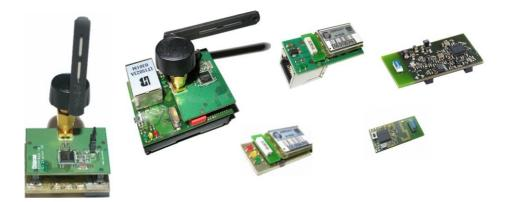
Figure 3: WeBee and EtherBee Module Family of CEESAR
